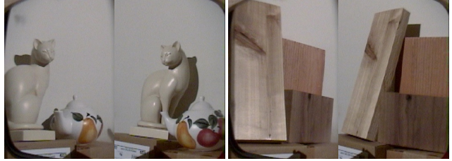
Figure 8: Sample stereo pairs for the two scenes used in our experiments. Note the specularities on the cat sculpture and the regions of uniform texture on the wood blocks, both of which make traditional spatial stereo matching difficult.
