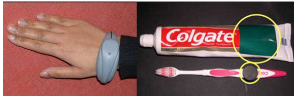
Figure 1: The iBracelet (left) and RFID tags (right)
