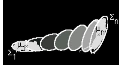
Figure 2: An example showing how the mean and covariance of the object (in this case a mouse) on the left is linearly interpolated into the mean and covariance of the object on the right, using our algorithm for linear interpolation. The leftmost ellipse corresponds to (\boldsymbol{\mu}_1, \Sigma_1) and the rightmost ellipse corresponds to (\boldsymbol{\mu}_n, \Sigma_n) . The affine prior \hat{\mathbf{a}} transforms any of these ellipses to the ellipse on its right.
