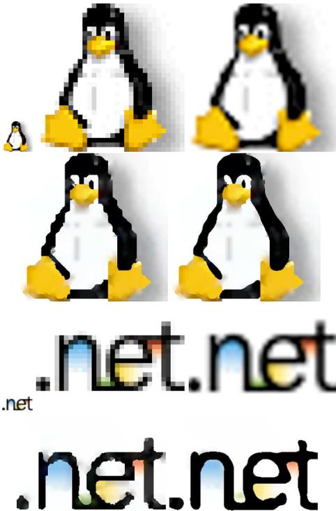
Figure 8. As a first step towards vectorization, the boundaries of the uniform zones have been smoothed with a spline. From left to right, the images are: the original icon, the nearest neighbor, the cubic interpolation, our interpolation without and with the spline
