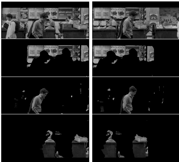
Figure 6: Notting Hill sequence. (Row 1) Original image pair of size 311 \times 552 , (Rows 2-4) Pixels assigned to warp layers 1-3 in I and I' .
