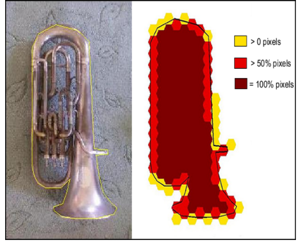
Figure 3. Different strategies for selecting “bubbles”. This particular examples shows a specific size of hexagon and translation, representing one user labeling. We can observe that the contour approximation depends on the strategy chosen. The polygon contour corresponds to the ground truth label from Caltech-101 [1].
