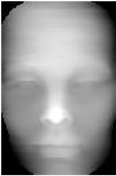
Figure 6. A depth map from the cyclopean viewpoint of the mannequin face in which light corresponds to near and dark to far.
