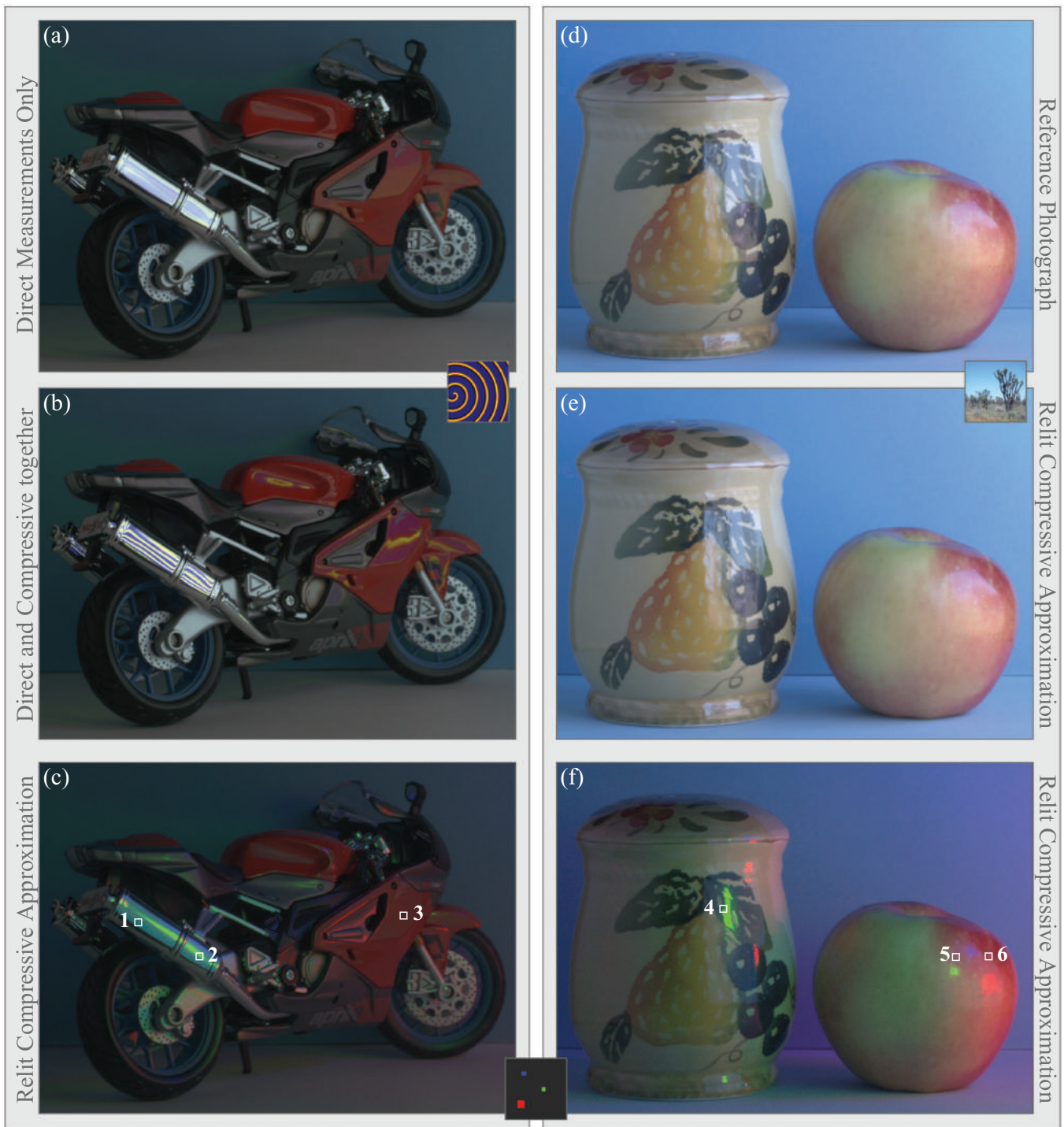
Fig. 11. Acquired reflectance fields. In the left column, a relit toy motorbike is shown. (a) and (b) are lit by the illumination condition shown in the inset; (a) only shows the effect of directly measured coefficients, while (b) also includes the coefficients obtained by compressive sensing; (c) the motorbike relit by three colored light sources. The right column shows a ceramic object and an apple. A reference photograph of the scene (d) lit by the illumination condition (shown in the inset) is compared to a computed result (e); (f) the scene under three small colored light sources. Reflectance functions of the six marked pixels are shown in Figure 12.
