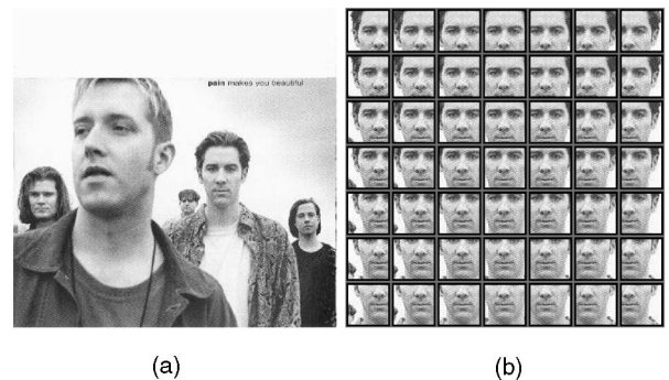
Fig. 16. (a) Test image. (b) Detection results. Different criteria lead to different detection results. Suppose all the subimages in (b) are classified as face patterns by a classifier. A loose criterion may declare all the faces as “successful” detections, while a more strict one would declare most of them as nonfaces.
