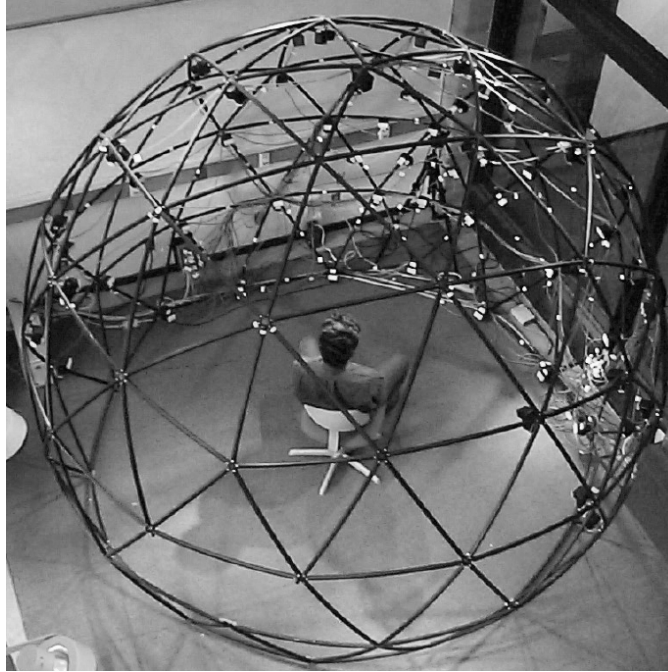
Figure 10: A geodesic dome with 64 strobes used to gather images under variations in illumination and pose.
