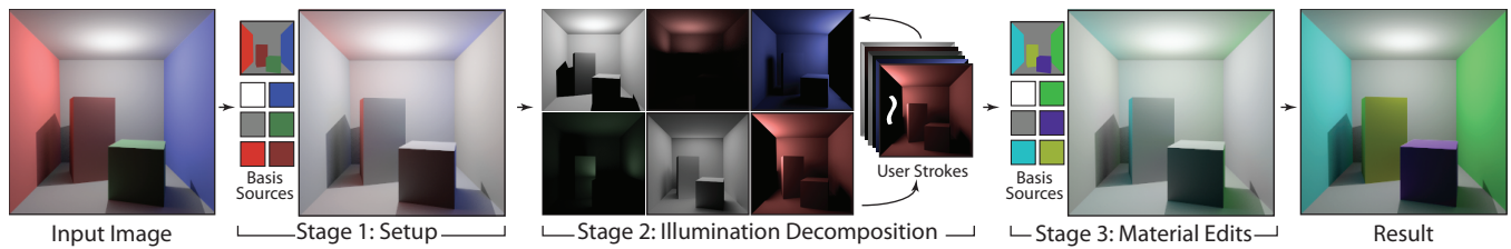
Figure 3: Our color editing system has 3 stages. We first compute intrinsic images using the approach of Bousseau et al., and sample the reflectance image to obtain basis sources. In the second stage we compute the illumination decomposition, with the user iteratively adding strokes to refine the result. In the final stage we modify the reflectance image and obtain a new set of basis sources, which is used with the decomposition to construct a new illumination image.
