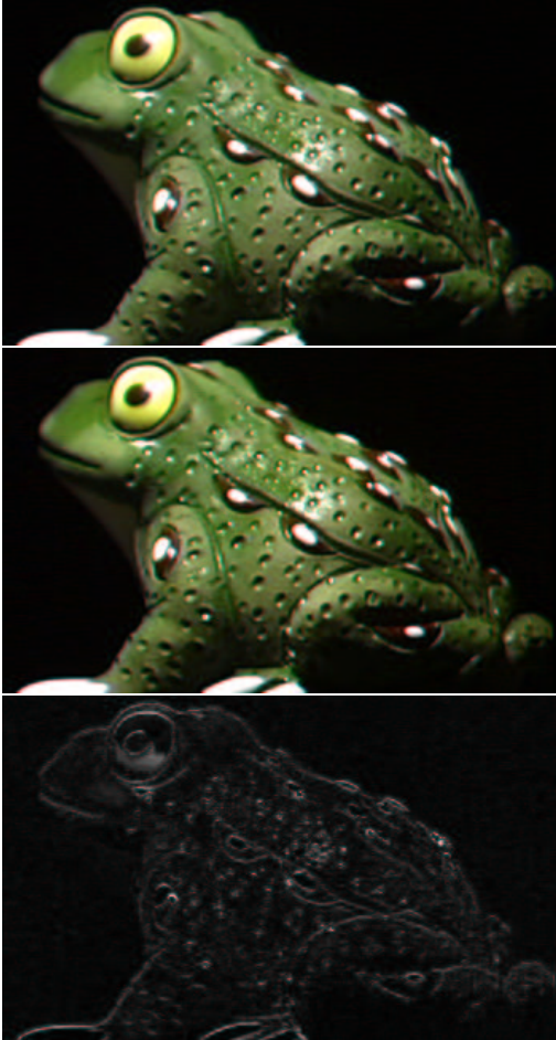
Fig. 6: Real image of a ceramic frog (top), rendered image of the ceramic frog using our image-based technique with a synthetic light source at the same location (middle), and the magnitude of the difference image between the real and rendered images (bottom).
