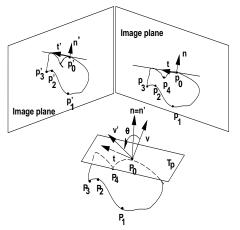
**Figure 3**. An illustration of motion in the tangent plane. Note that the point  $p'_4$  corresponding to the viewing direction  $\mathbf{v}'$  has been omitted deliberately because such points are good candidates for self-occlusion.
