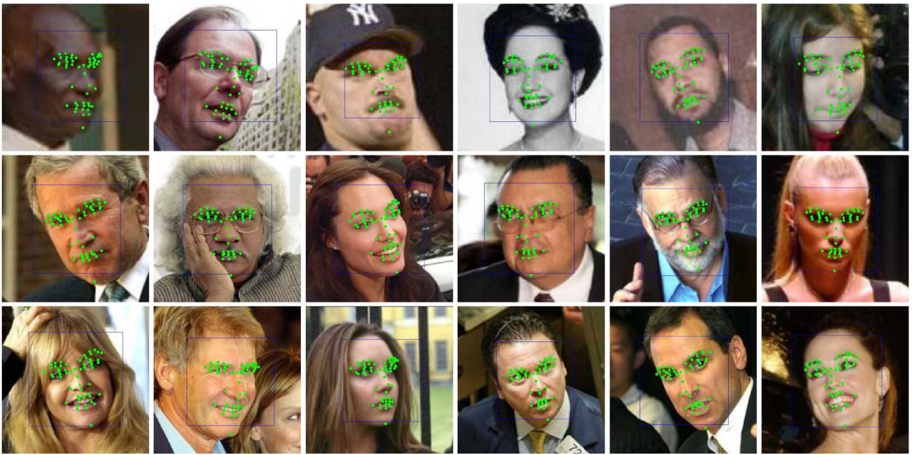
Fig. 7. Images from Labeled Faces in the Wild (LFW), along with OpenCV face detections (blue rectangles) and 55 parts localized by our detector (green dots). Our mean accuracy is 5.18 percent of the interocular distance.
