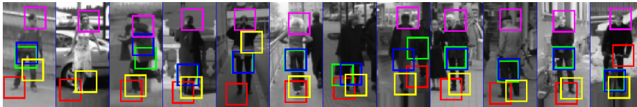
Fig. 1. Response of first 5 learned components classifiers on randomly selected INRIA pedestrian test images (best viewed in color). At most one box is displayed per component after non-maximal suppression and thresholding. Three components correspond to semantically meaningful parts (head-magenta, left foot-red, right foot-yellow); 2 correspond to the region between between the legs. The components were learned with no component labels provided during training. See Sec. 4.3 for details.
