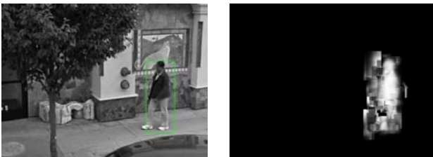
Figure 4. Pedestrian detection algorithm results: (left) Bounding box and (right) per-pixel probability map
