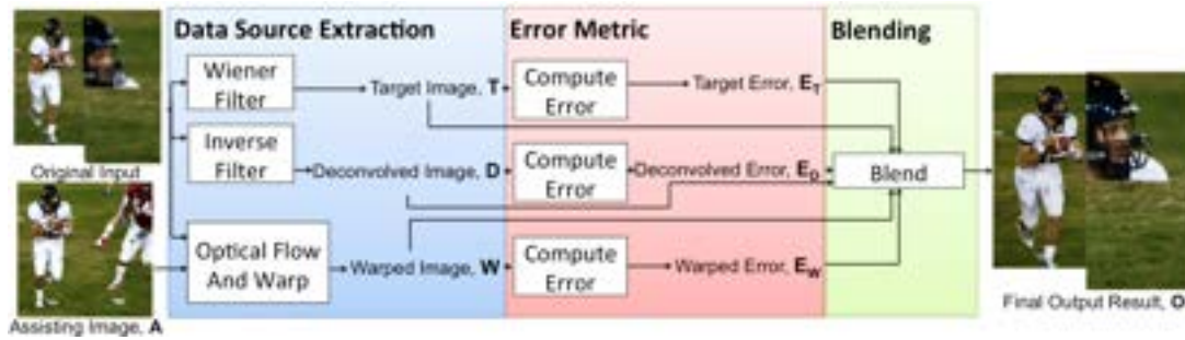
Figure 2: Pipeline for our method. Our algorithm takes two inputs, the blurry image to sharpen and a similar but sharp assisting image(s). We sharpen the input using a conservative Wiener filter to obtain a baseline target T , and apply an aggressive inverse deconvolution filter to obtain D . We also use optical flow and warping to get W from the assisting image. With the three registered data sources, T , D , and W , we compute their errors: E_T , E_D , and E_W . We then blend to produce output O .
