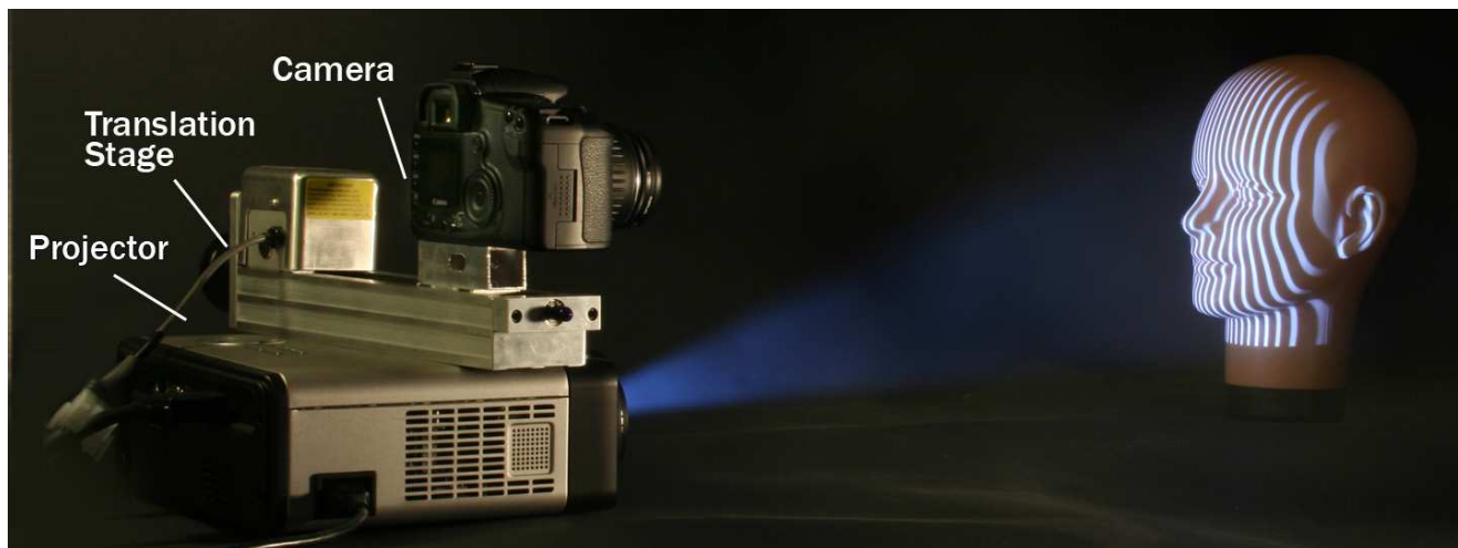
Figure 9: Capture rig used for viewpoint coding experiments. A digital camera is moved to the different required positions using a translational stage, while structured illumination is provided using a projector.
